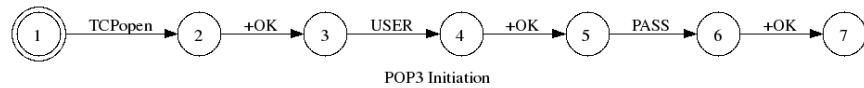
Figure 4.6: POP3 Session Initiation - POP3 session initiation starts with the TCP connection from the client to the server. The server replies with +OK then the client attempts authentication with USER then PASS commands.
